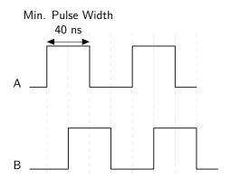
Figure 5: AquadB signals and minimum pulse width
