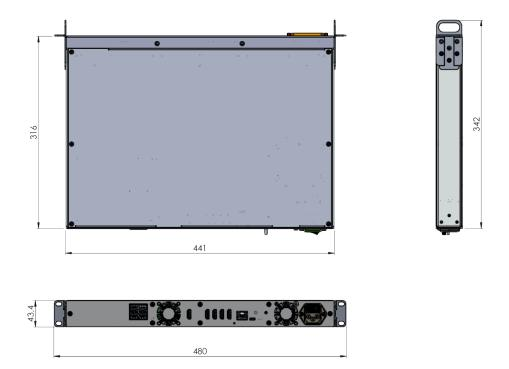
Figure 11: ACQ2206 Channel Panel Case Dimensions (mm)
