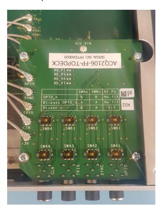
Figure 3: Top Deck Switches
