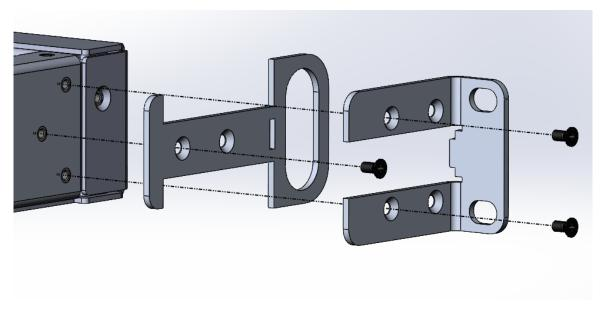
Figure 9: Channel Panel Case Rack Mount
