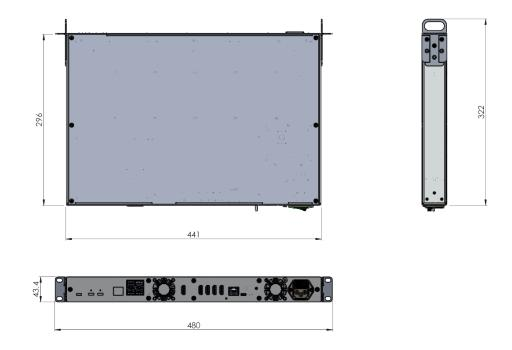
Figure 10: ACQ2206 Standard Case Dimensions (mm)
