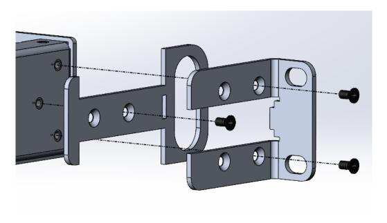
Figure 8: Standard Case Rack Mount
