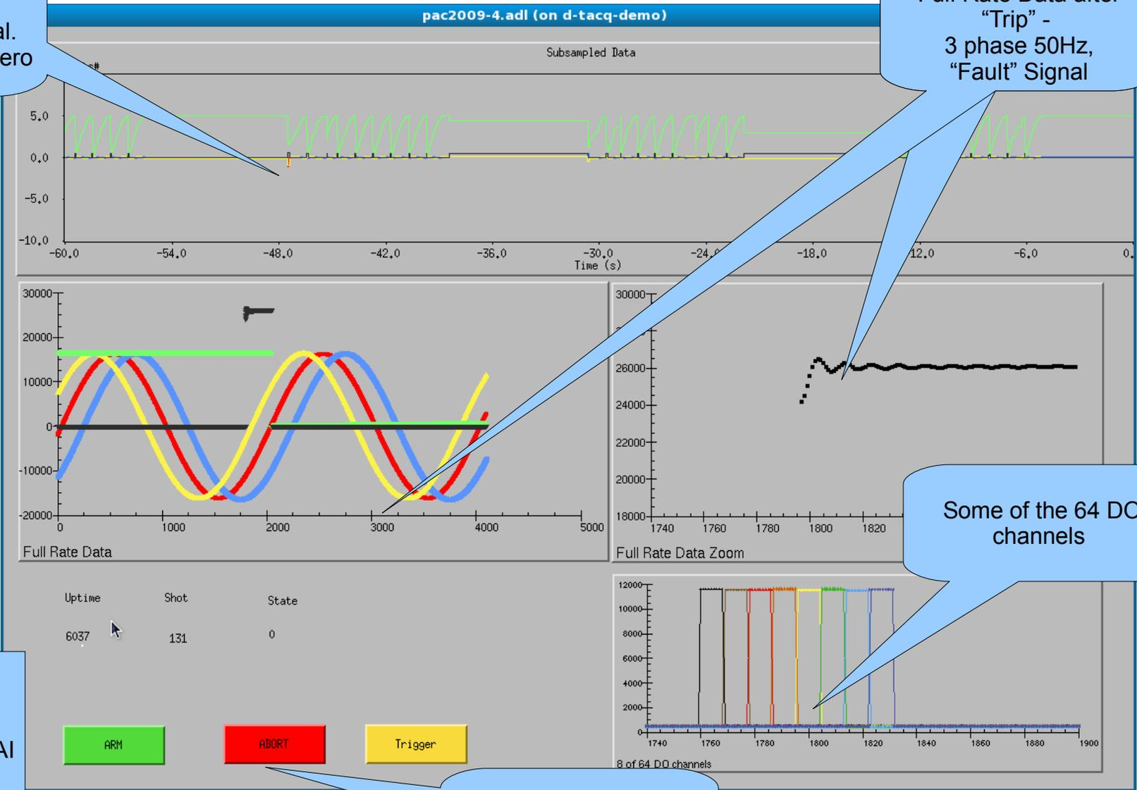
Full Rate Data after "Trip" - 3 phase 50Hz, "Fault" Signal
