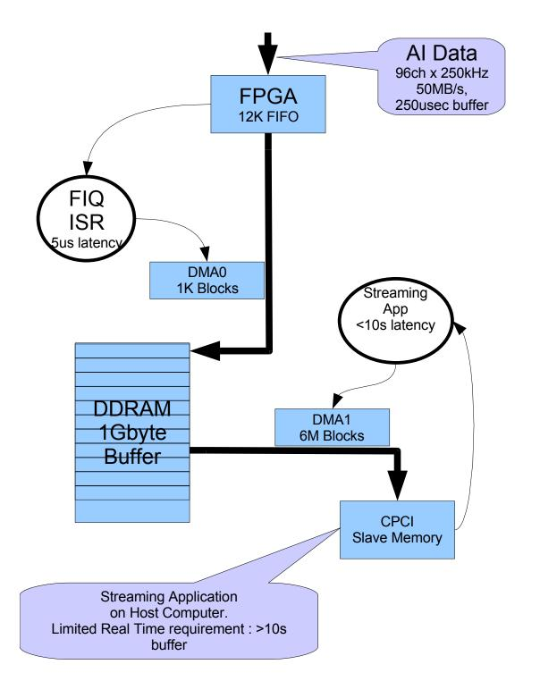
• CPCI backplane operation already used extensively for PCS. PCS applications are optimised for Latency. • High bandwidth CPCI backplane also suitable for continuous data streaming for diagnostic applications, where the on-board DDRAM is no longer big enough to hold all the data.
