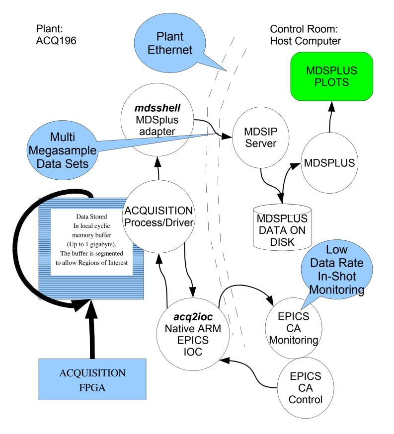
Embedded MDSplus "ThinClient" - store calibrated data direct to MDS server Inot shown] Embedded MDSIP allows MDSplus server to control digitizer. And, via the system slot function, it's possible to control other devices in the chassis.
